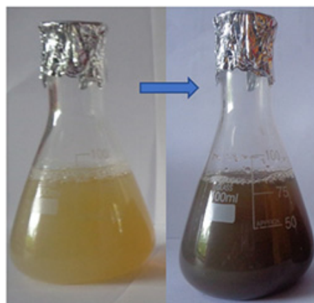
Fig. 1 Visible colour change of Datura metel leaf extract after silver nanoparticles synthesis
